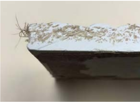
Plaster sample with gypsum and coconut fibers
